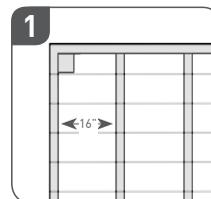
**1 16" BASIC INSTALLATION SUBSTRUCTURE**
