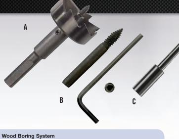
One-piece construction bits with cutter blades welded to shanks. They are self-feeding with one replaceable pilot screw that fits all sizes, eliminating the need to match parts. The black oxide finish is rust resistant. The easy to use, fast cutting bits won't separate when backing out, and they're easy to sharpen with only two cutters.
