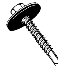
#12-14 x 1-1/4" HWH w/1-1/8" Oversize Bonded Washer (pre-drilling w/oversize holes required) Figure 15c
