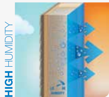
Increases permeability in summer to let moisture escape when needed.
